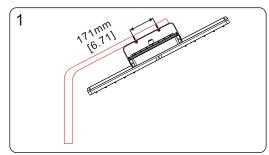
1. Drill 2x Ø15 holes for fixing screws
