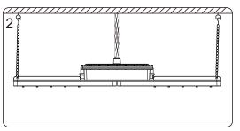
2. Fix the hanging chain to light fixture. Wire the cable through the metal conduit and then connect it with the power.
