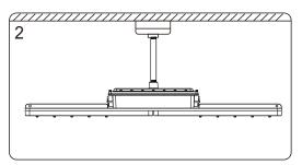
2. Wire the cable to enclosure of junction box and install the pole to junction box.
