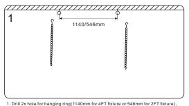
1. Drill 2x hole for hanging ring(1140mm for 4FT fixture or 546mm for 2FT fixture), and fixing them.
