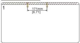
1. Drill 2x Ø15 holes for expanded screws, and fixthem to the ceiling.
