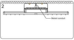
$2. \ \mbox{Install}$  the fixture to the expanded screws, and tighten the nuts. (Metal conduit need to apply here)
