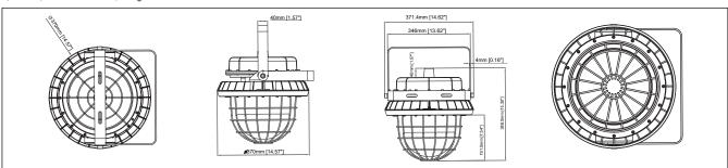
This structure type with bracket, global glass lens and wireguard to generate 180° light distribution. We also can put corn bulb In the global glass lens to make this beam angle up to 360°.
